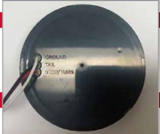
FIGURA 6 - LUZ LED FINAL INSTALADA
