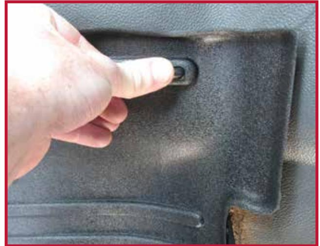
15. For optimal adhesion do not disturb the hook for a period of 20 minutes after installation.
