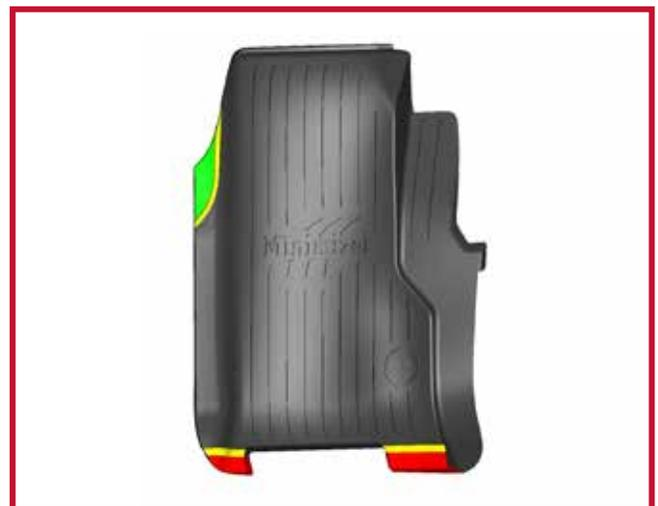
Use a sharp utility knife as shown in Figure 10 to trim along the outside edge of the rib preserving the rib for liquid containment.
