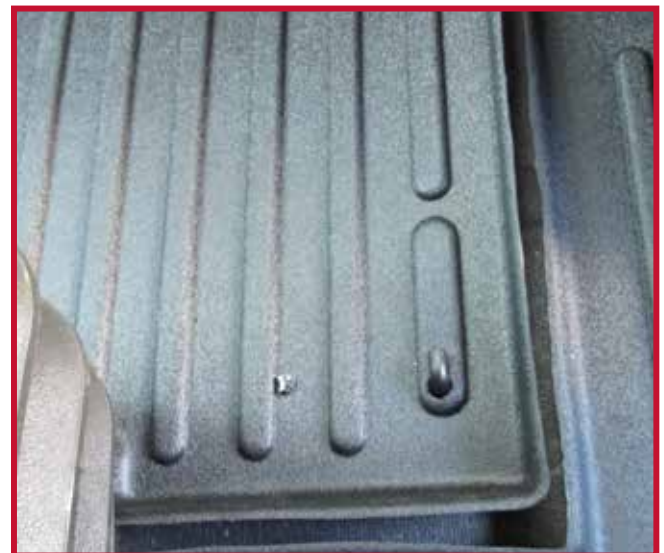
Figure 8 - Driver Mat Hook Installation
