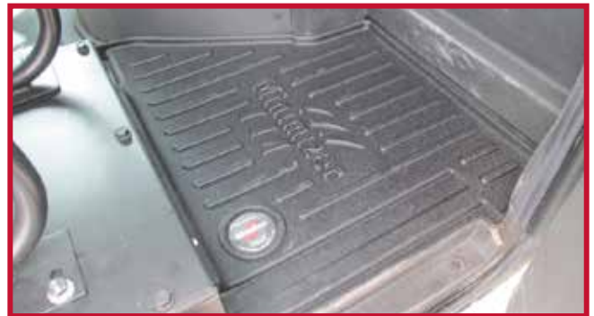
Figure 9 - Passenger Mat Installed
