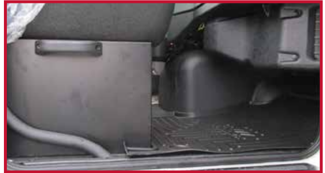
Figure 22 - Fixed Base Passenger Seat with Trimmed Mat
