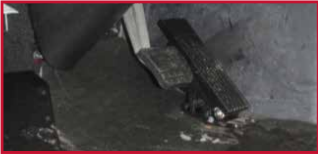
Figure 2 - Floor Mounted Throttle Pedal Mechanism
