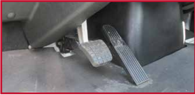
Figure 2 - Floor Mounted Throttle Pedal Mechanism
