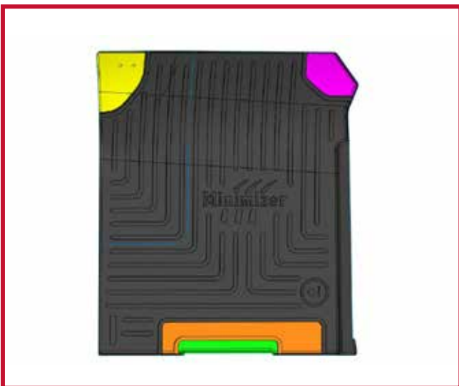
Figure 21 - Passenger Mat Trimming Diagram
