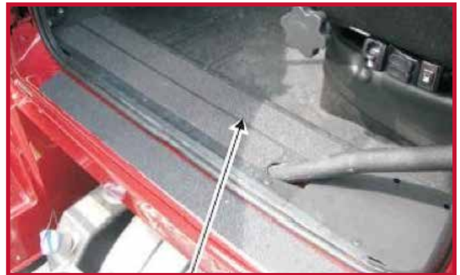
Figure 6 - Driver Side Electrical Tray
