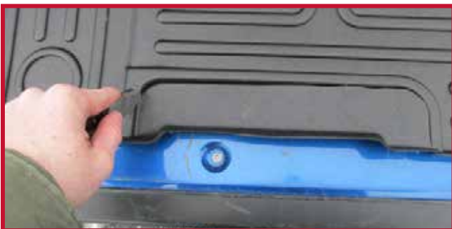
Figure 16 - Hand Trimming for Seat with Rubber Boot
