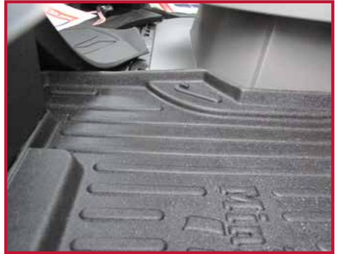
Figure 9 - Passenger Mat Retention Hook Location
