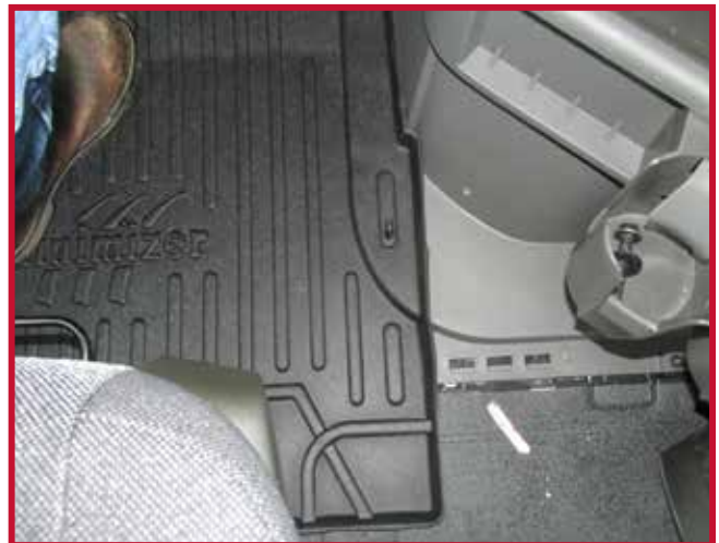
Figure 7 - Driver Mat Hook Installation
