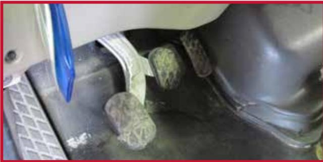
• Kit #10002743 shown in Figure 3 is compatible with 1996-2009 Sterling/Ford Models with a suspended throttle pedal and a floor mounted brake pedal as shown in Figure 4.
