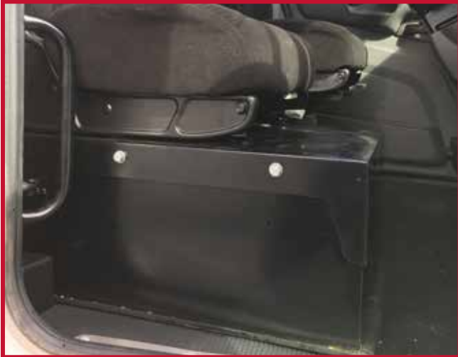
Figure 8 - Battery Box Passenger Seat Base
