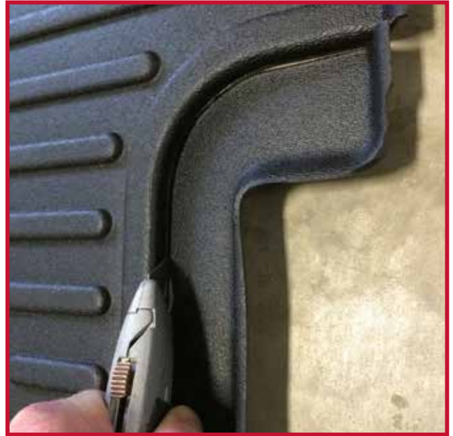
Figure 8 - Trimming for Aftermarket Seats
