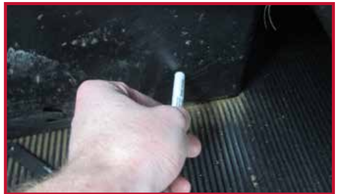
Figure 11 – Apply Primer to Seat Base
