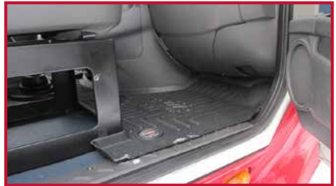
Figure 9 - Passenger Mat with Fixed Seat
