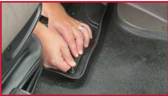
Figure 7 - Apply Pressure to Hook
