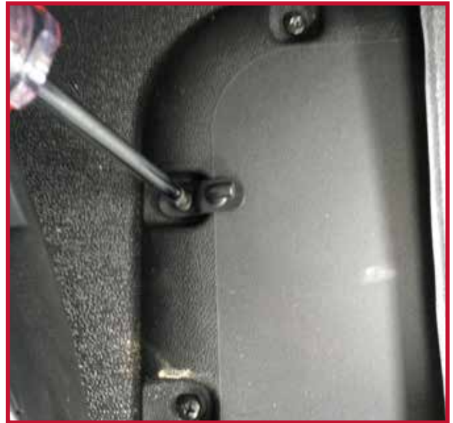
Figure 8 - Retention Hook Installation
