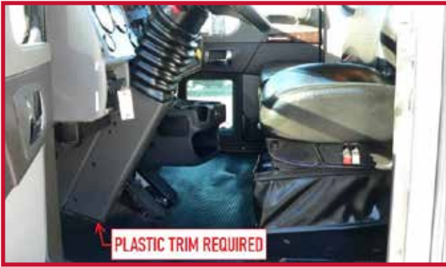
Figure 9 - Steering Column Fitment
