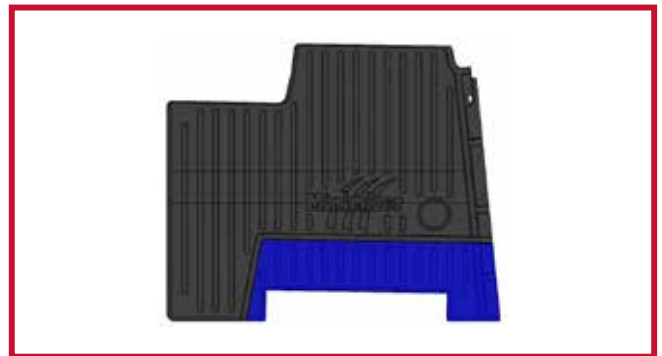
Figure 12 – Passenger Mat Trimming Diagram for kits 105187, 105189, 105191 & 105193
