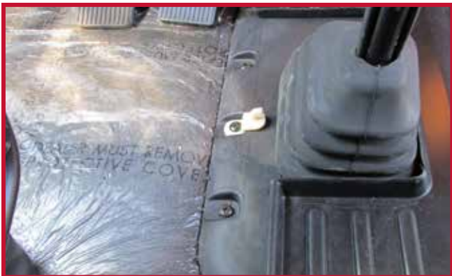
Figure 13 - Proper Hook Orientation
