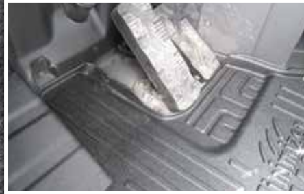
Figure 3 - Driver Mat Contact with Kick Panel
