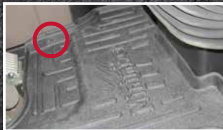
Figure 5 - Opening Location for Retention Hook
