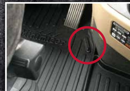
Figure 11 - Driver Mat Hook Installation
