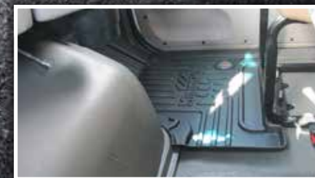
Figure 13 - Passenger Mat Hook Installed on Doghouse Trim
