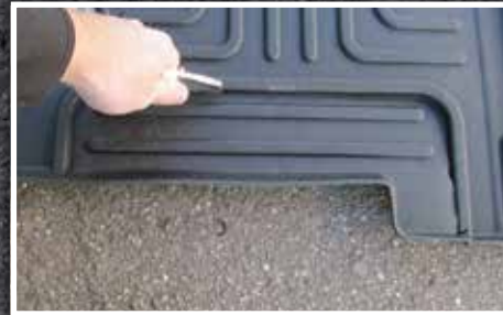
Figure 8 - Trimming for EzyRider Seat
