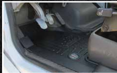
Figure 7 - Driver Mat Installation with EzyRider Seat
