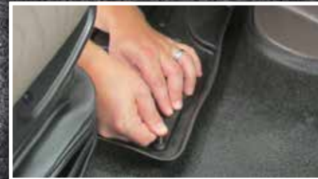
Figure 11 - Properly Installed Driver Mat and Hook
