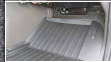
Figure 12 - Properly Installed Driver Mat and Hook
