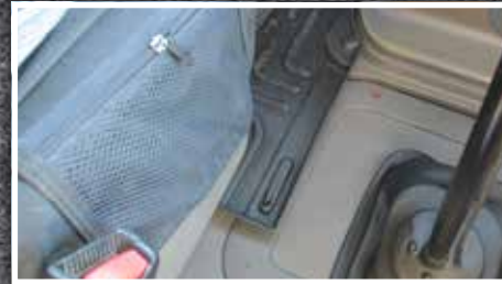
Figure 10 - Driver Mat Hook Installation
