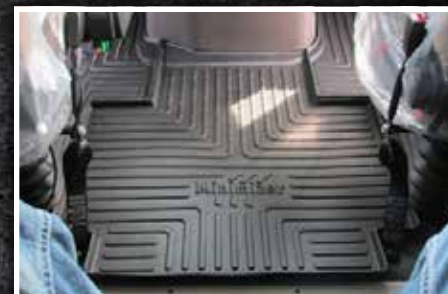
Figure 8 - Center Mat Installed
