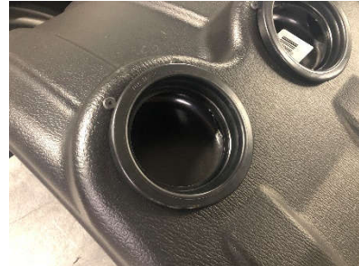
FIGURE 4 – FENDER WITH RUBBER GROMMET.
