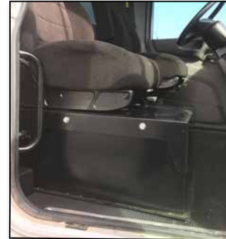
Figure 8 - Battery Box Passenger Seat Base
