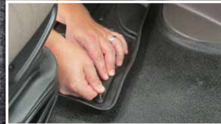
Figure 7 - Apply Pressure to Hook
