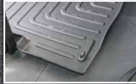
Figure 6 - Confirm Location Driver Mat and Hook
