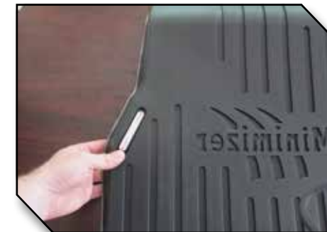
Figure 10 - Hook Inserted in Driver Mat
