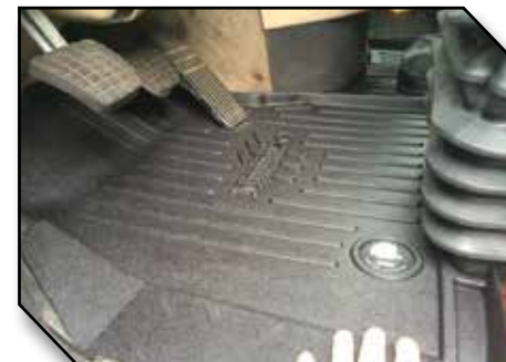
Figure 8 - Driver Mat Fit After Trimming
