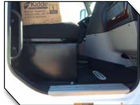
Figure 6 - Passenger Seat with Under Seat Battery Storage
