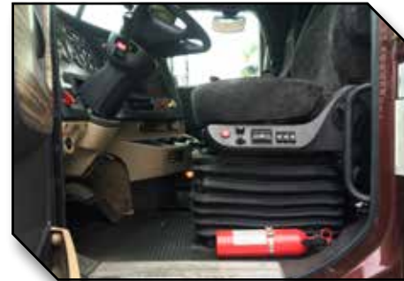
Figure 5 - Driver Seat with Rubber Skirt
