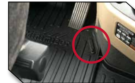
Figure 11 - Driver Mat Hook Installation
