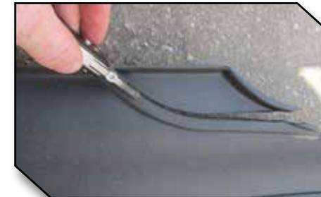
19. The passenger floor mat is designed to accommodate fixed seats, bench seats and suspension seats. For trucks equipped with a partial or full width bench seat the rear portion of the passenger mat will need to be trimmed. The area to trim is shaded in red on Figure 9 and a raised trim line (shaded yellow) has been provided to use as a guide. Figure 11 below shows the fit of the passenger mat when properly trimmed to for a bench seat.
