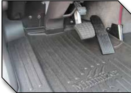
a) For Freightliner models M2 112, 108SD and 114SD a small portion of the right side of the driver mat must be trimmed away in order to fit safely around the dog house trim panel. There is a raised rib molded into the driver mat to contain liquid and act as a trim guide. See the red shaded area in Figure 5 to identify the portion to trim.
