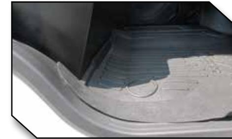
20. Move the accelerator, brake, and clutch pedals through their full range of motion to confirm there is no interference with the Minimizer floor mat.
