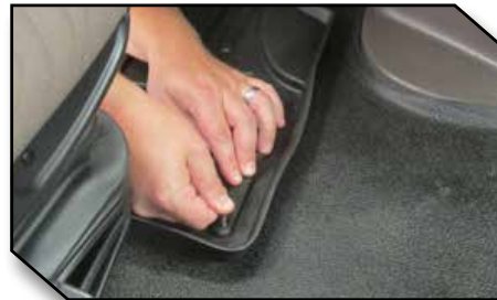
Figure 7 - Apply Pressure to Hook
