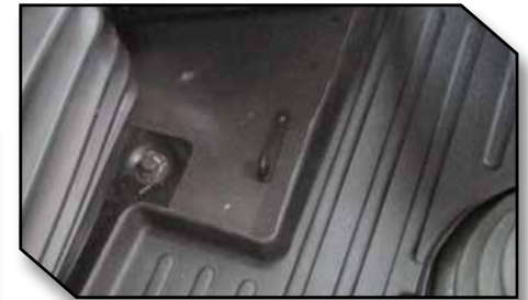
Figure 8 - Properly Installed Retention Hook
