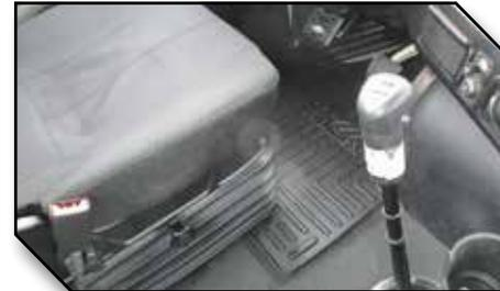
9. Mark the approximate position where the hook needs to be attached to the floor. Once the position is located, remove the driver mat from the truck.
