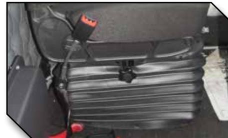
Figure 11 - Hand Trimming for Seat with Rubber Boot
