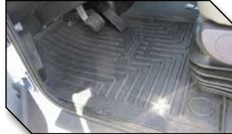
Notes: The driver mat is designed to fit several common OEM seat bases. Truck seats that are equipped with a large rubber boot around the seat suspension (as shown in Figure 10) will require hand trimming at the time of installation. Some other aftermarket seats may also require hand trimming for proper fit. There is a raised rib molded into the driver mat to use as a trim guide and to contain liquid. Use a sharp utility knife to trim the mat as shown in Figure 11.
