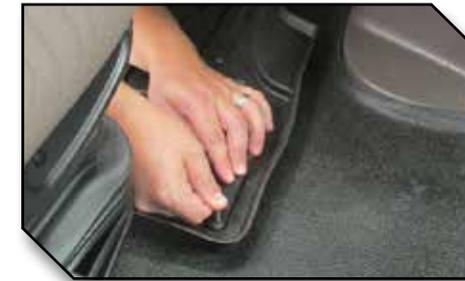
15. Position the passenger floor mat in the truck. Make sure the passenger mat is pushed all the way forward so the outside lip makes full contact with the doghouse trim panel and fire wall as shown in Figure 15.
