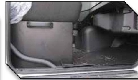
16. Use the same process listed in steps 7-14 above to attach the passenger mat retention hook to the floor. For trucks with carpeted floors install the hook to interior trim at the right front corner of the passenger side. There is a small oval shaped trim line visible on the outside perimeter of the mat where the hook opening should be trimmed. Follow the same basic steps to prime the steel surface and attach the hook to the cab.
