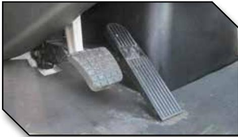
Figure 2 - Floor Mounted Throttle Pedal Mechanism
