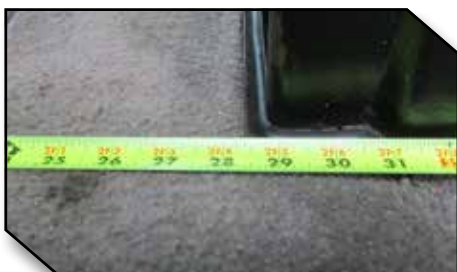
Figure 2 - 28.75” Measured at Front of Seat Base
