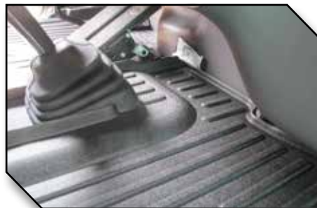
Figure 8 - Fit After Trimming
