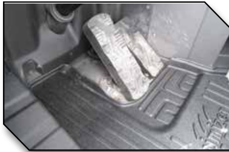
Figure 3 - Driver Mat Contact with Kick Panel
