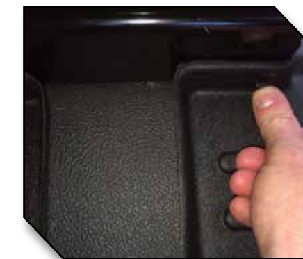
Figure 10 - Apply Pressure to Hook
