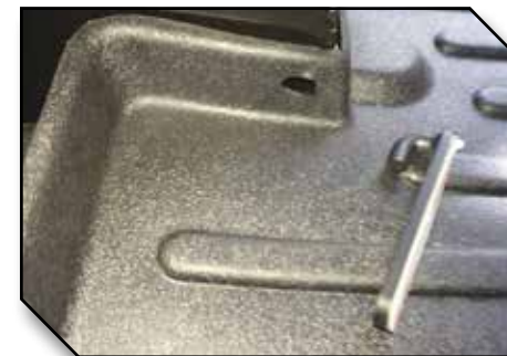
Figure 9 - Driver Mat with Hook Opening
