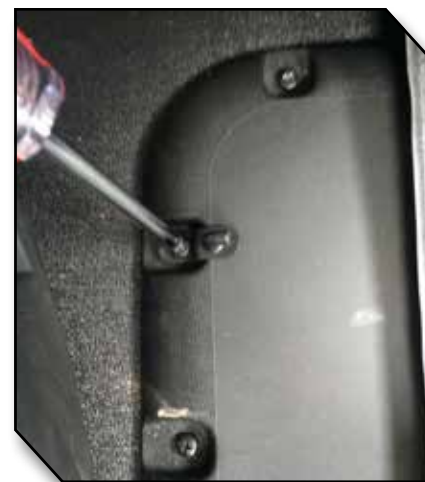
Figure 7 - Retention Hook Installation
