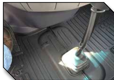
Figure 8 - Kit FKPCR1MB Driver Mat with Retention Hook
