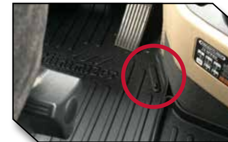
Figure 11 - Driver Mat Hook Installation
