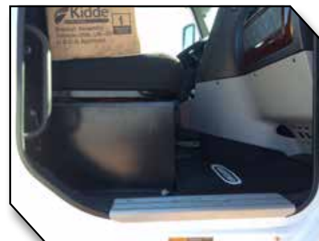
Figure 6 - Passenger Seat with Under Seat Battery Storage
