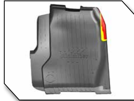
Figure 5 - Driver Mat Trimming Diagram
