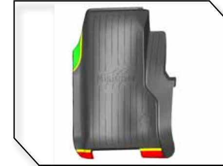
Figure 9 - Passenger Mat Trimming Diagram
