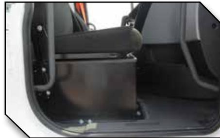
**Figure 5 - Center Mat Trimming for Battery Box**
