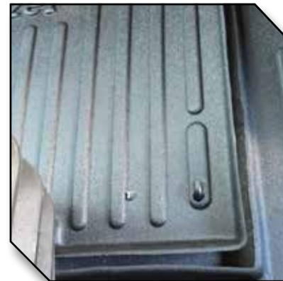
18. Pull the driver mat toward the rear of the truck to confirm that the hook is fully engaged into the mat and that the hook is adhered to the floor. If the hook is not functioning properly or the mat cannot be securely installed, do not use a Minimizer floor mat on the driver side of the vehicle.
