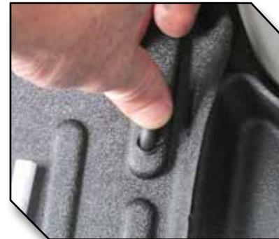
17. For optimal adhesion do not disturb the hook for a period of 20 minutes after installation. Figure 8 below shows the properly installed driver mat and hook.
