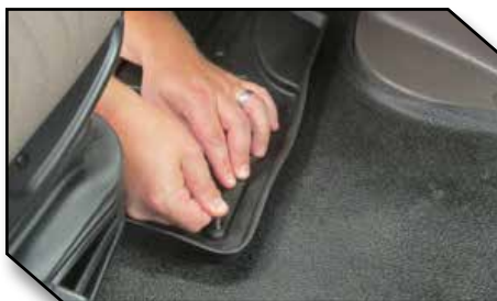
Figure 7 - Apply Pressure to Hook
