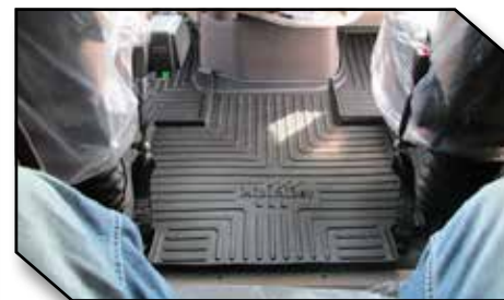
Figure 8 - Center Mat Installed
