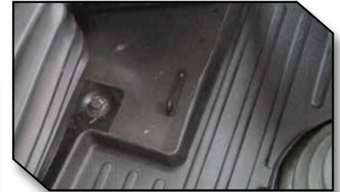
Figure 8 - Properly Installed Retention Hook
