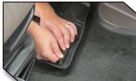
Figure 7 - Apply Pressure to Hook
