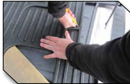
**Note:** Figure 5 below shows the center mat from kit FKFRTLASCMB installed in a day cab truck. This mat was trimmed to fit around the existing fire extinguisher and DOT roadside safety kit.
