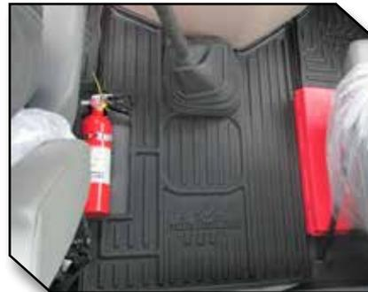
6. Straighten the rubber boot that surrounds the gear shift so it rests smoothly on top of the center mat as shown below in Figure 6.
