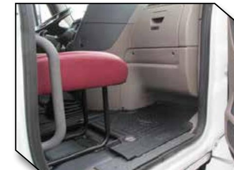
20. Pull the driver mat toward the front of the truck to confirm that the hook is fully engaged into the mat and that the hook is adhered to the floor. If the hook is not functioning properly or the mat cannot be securely installed, do not use a Minimizer floor mat on the driver side of the vehicle
