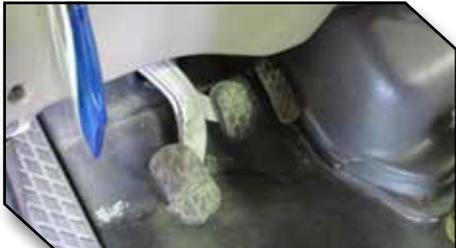
• Kit FKST2B shown in Figure 3 is compatible with 1996-2009 Sterling/Ford Models with a suspended throttle pedal and a floor mounted brake pedal as shown in Figure 4.
