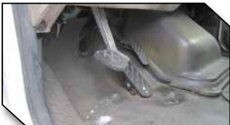
• Kit FKST3B shown in Figure 5 is compatible with 1996-2009 Sterling/Ford Models with floor mounted throttle pedal and floor mounted brake pedal as shown in Figure 6.
