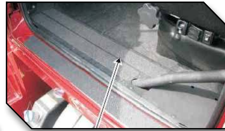
Figure 4 - Driver Side Electrical Tray
