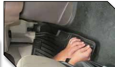
Figure 11 - Passenger Mat In Position
