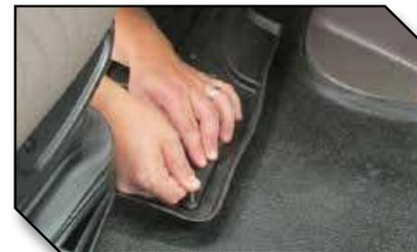
15. Position the passenger mat in the truck. Make sure the passenger mat is pushed all the way forward so the outside lip makes full contact with the doghouse trim panel and fire wall.
