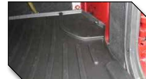
17. Confirm that the retention hook is fully engaged into the driver mat and that the hook is adhered to the floor. If the driver mat hook is not functioning properly or the mat cannot be securely installed, do not use a Minimizer floor mat on the driver side of the vehicle.
