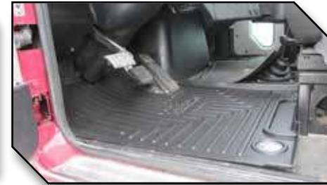
• The driver mat must be pushed all the way forward so the front lip is making full contact with the doghouse trim panel and fire wall.
