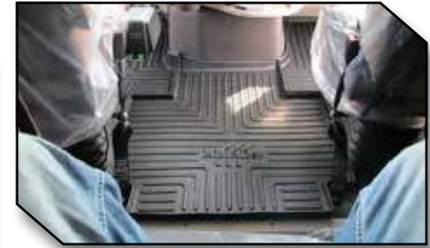
Figure 8 - Center Mat Installed
