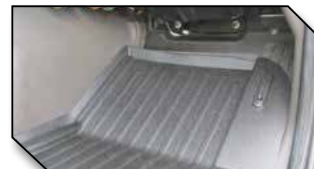
Figure 12 - Properly Installed Driver Mat and Hook
