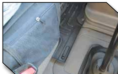
Figure 10 - Driver Mat Hook Installation
