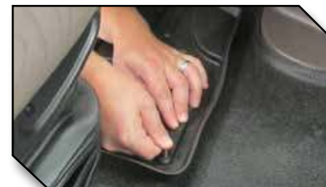
Figure 11 - Properly Installed Driver Mat and Hook
