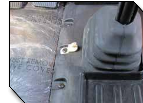
Figure 14 - Proper Hook Orientation
