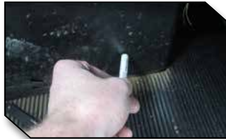
Figure 11 – Apply Primer to Seat Base
