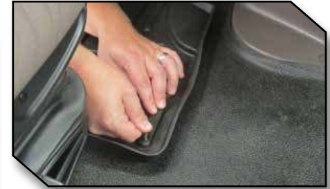
Figure 7 - Apply Pressure to Hook
