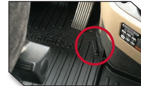
Figure 11 - Driver Mat Hook Installation
